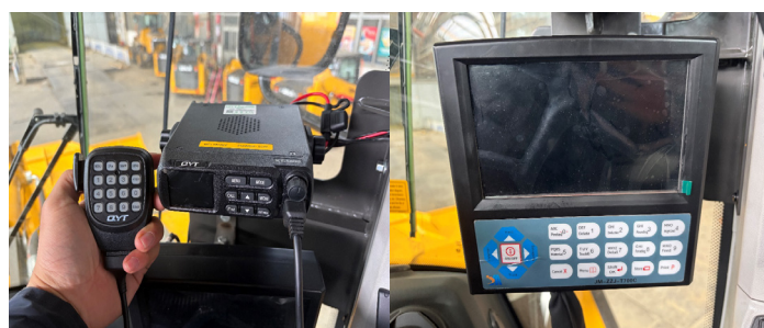
Intercom System & Intelligent Weighing System
